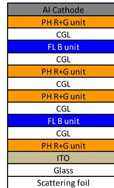
Figure 1. Brite1 white OLED stack
