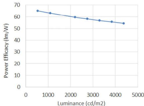
**Figure 9: Efficacy vs. luminance for 2X amber OLEDs**
