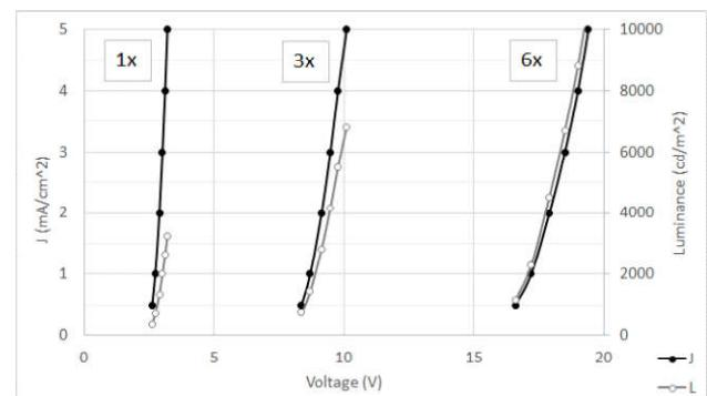
Figure 2: J-V-L curves for 1X, 3X and 6X OLEDs
