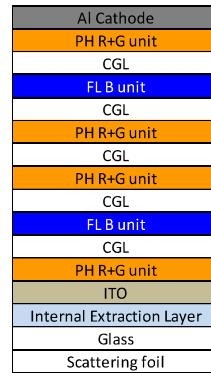
**Figure 5:** Brite2 white OLED stack
