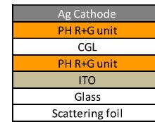
**Figure 8:** High-efficiency 2X amber OLED
