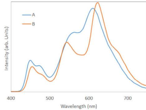
**Figure 4:** Spectral comparison for standard white stack (A) and improved CRI white stack (B)
