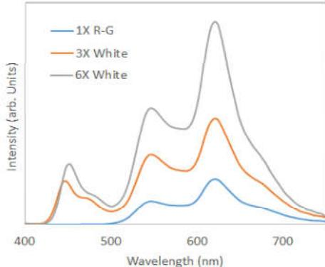
**Figure 3:** EL spectra for 1X, 3X, and 6X OLEDs
