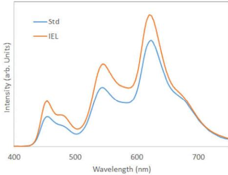
**Figure 6:** Spectral comparison for 6X white on standard and IEL substrates
