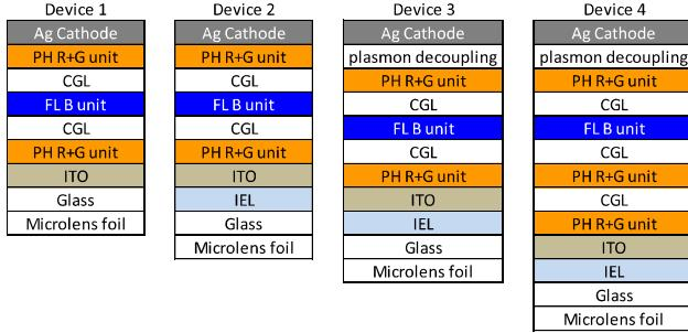
**Figure 7:** Experimental 3X and 4X white OLED stacks
