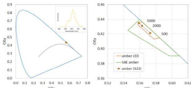
**Figure 10: Color and EL spectrum for 2X amber OLEDs**
