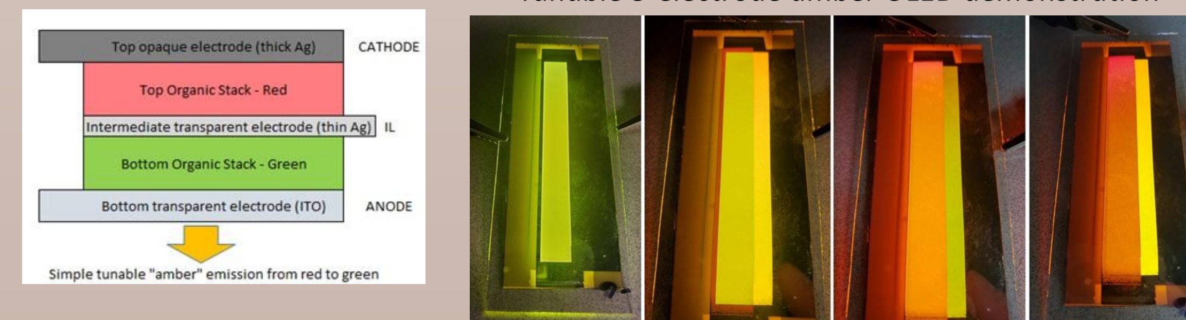
CCT range tunable by adjusting charge balance between Blue-Yellow stacks
